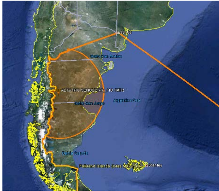
Figure 2 – Designated operational coverage limited to the boundaries of the FIR Commodore Rivadavia in Argentina; (FIR-U on 118.100 MHz)
